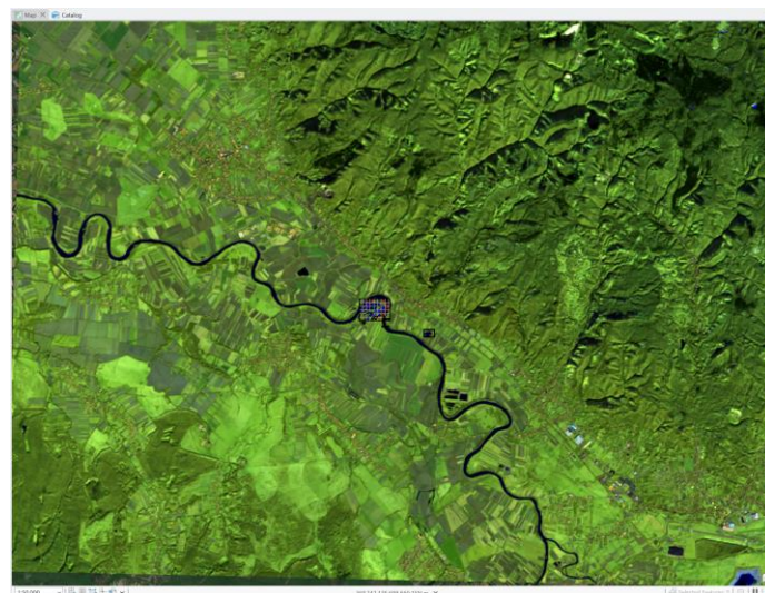
Fig.3. False Color Urban Composite [4] - Based on bands B12, B11, B4
