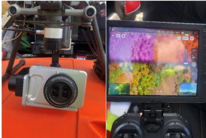
Fig.2. Agrowing multispectral lens equipped on a DJI M200 UAV
