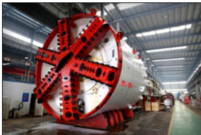
Fig.10. An EPB TBM by Terratec [12]
