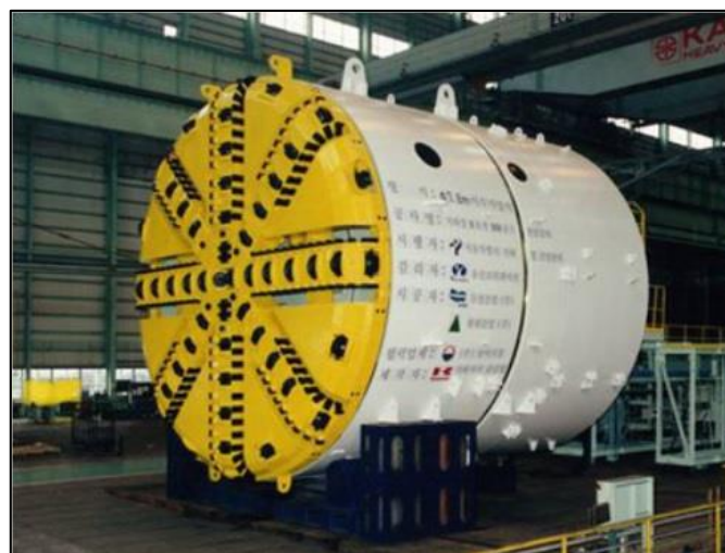
Fig.9. A Slurry Shield TBM by Mitsubishi [11]
