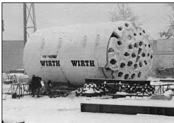
Fig.6. An open-face gripper shield TBM by Wirth [3]
