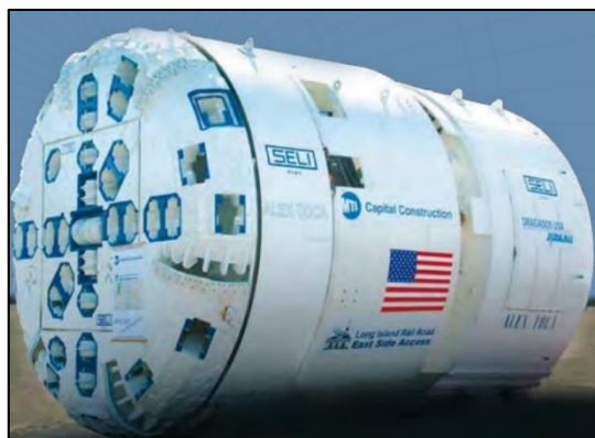
Fig. 7. A Double Shield TBM by Seli [8]
