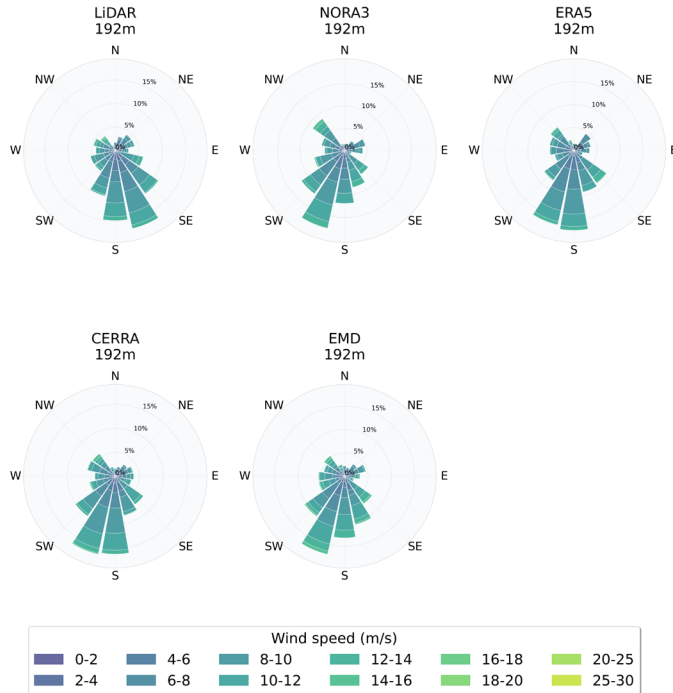
Fig. 4. Wind rose comparison between LiDAR measurements and reanalysis models at 192 m.
