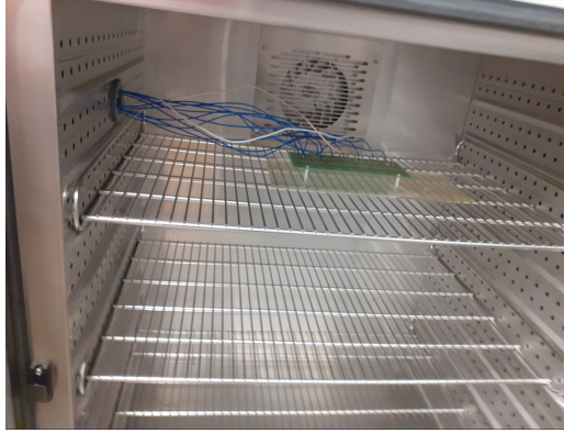
Fig. 2. Image of the test board inside the chamber.
