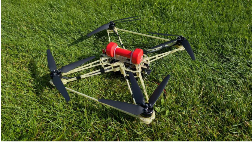
Fig. 6. UAV platform used for hover-mode validation with the tested lithium-ion battery pack.
