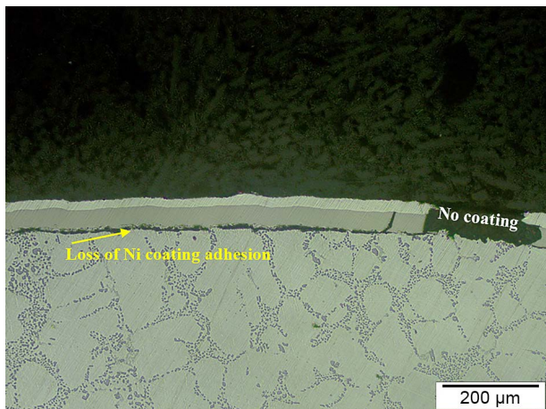
Fig. 4. Coating defects on sample 1: missing coating and loss of Ni coating adhesion, non-etched state
