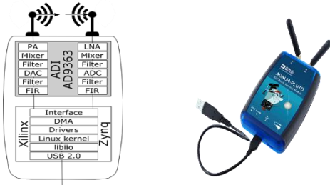
Figure 1: ADALM-PLUTO detailed component view
