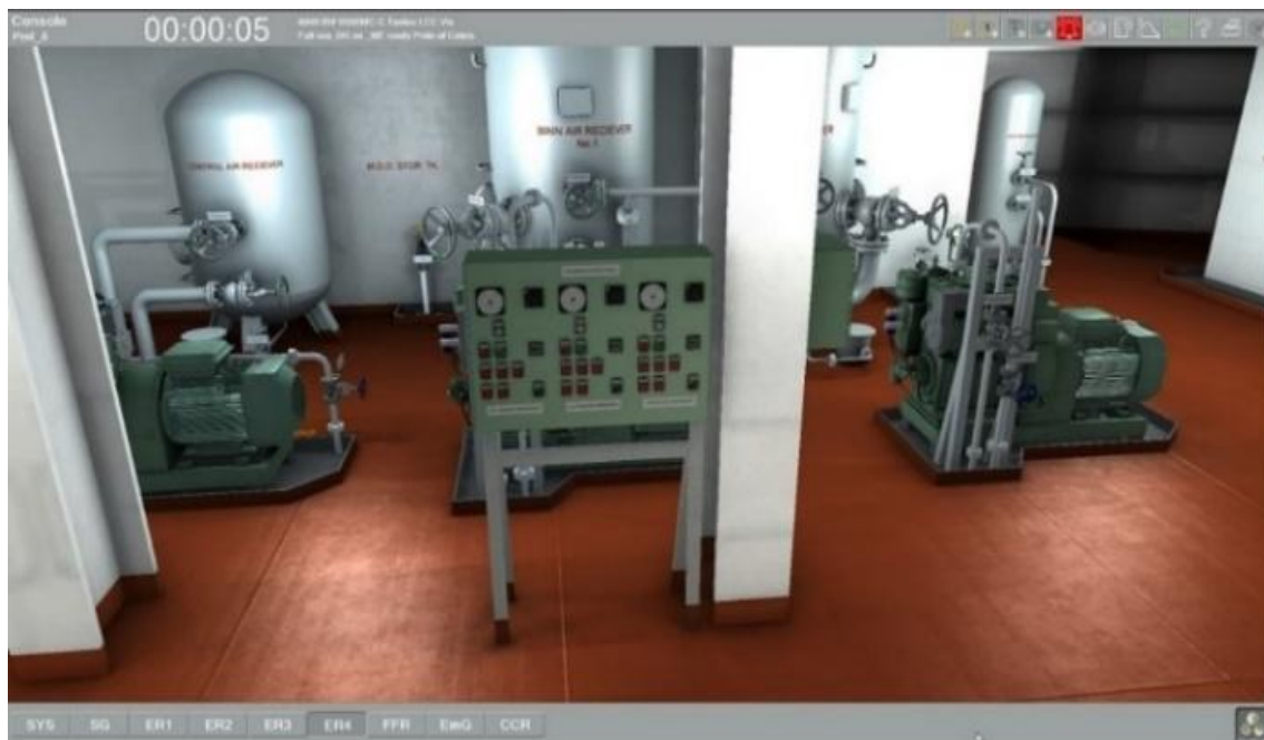
Figure 2: Tridimensional (3D) view and operation for simulated equipment
