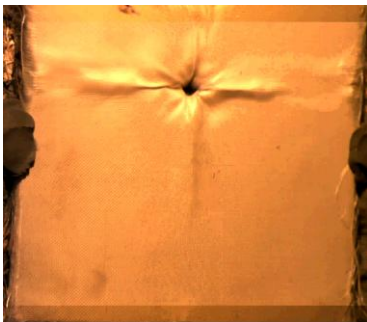
d) perforation of first layers (stage I)
