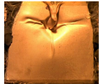
f) bullet rebound and partial shape recovery of the panel (stage III)
