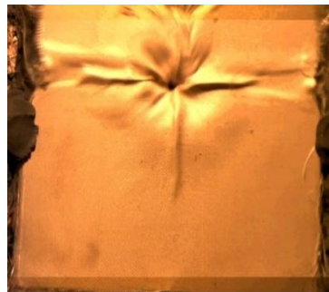
e) deformation of layers (stage II)
