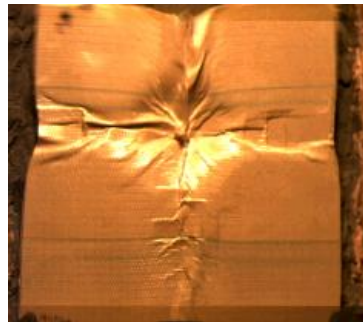
b) deformation of layers (stage II)
