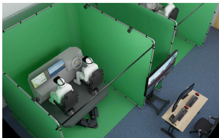
Figure 10: Mixed reality (MR) simulator for fast boats – MBNA project
