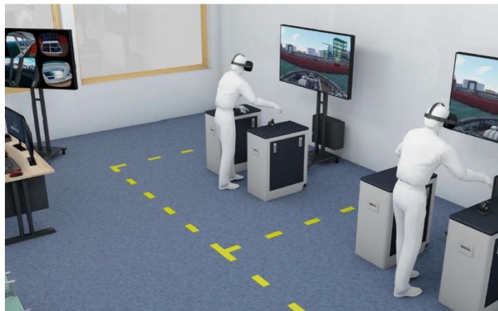
Figure 7: Virtual reality (VR) simulator for tug manoeuvring – MBNA project
