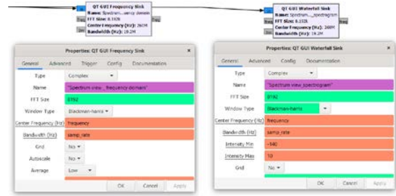
Figure 4: Configuration of frequency domain and spectrogram spectrum display settings
