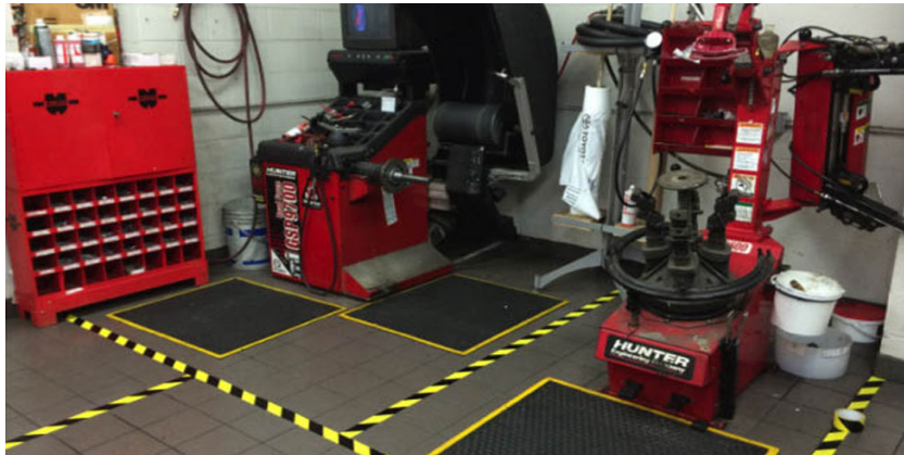
Figure 3: Warning markings for high risk areas[3]
