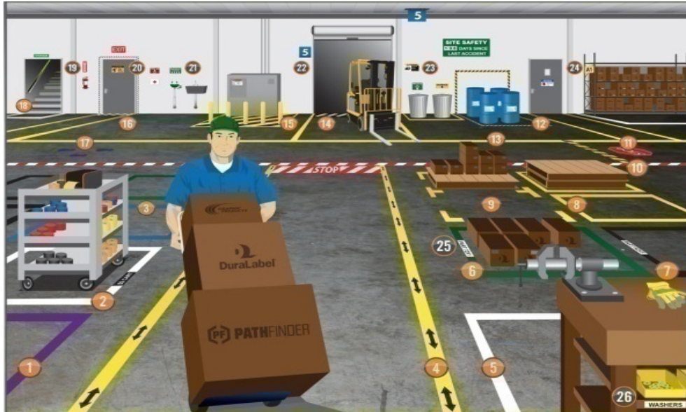
Figure 2: Markings for delimiting areas in a hall [2]
