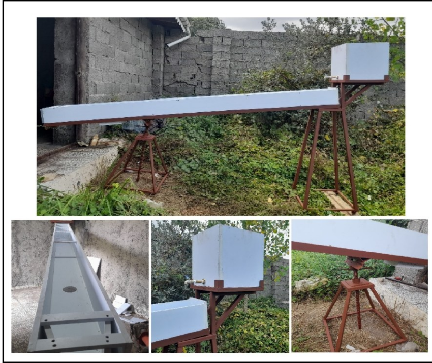
Fig. 3. Experimental setup of the hydraulic flume used to measure soil detachment capacity ( D_c ). The system includes a water supply tank, adjustable slope channel (3 m length, 0.2 m width), and a circular sample holder (0.1 m diameter) installed near the downstream section for testing soil samples under controlled overland flow conditions.
