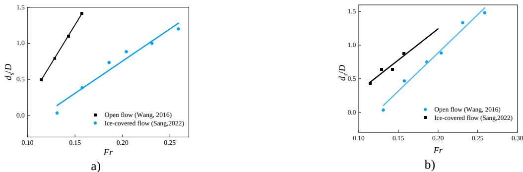
Fig. 13. Influence of flow Froude numbers on the scour depth: a) front pier; b) rear pier.
