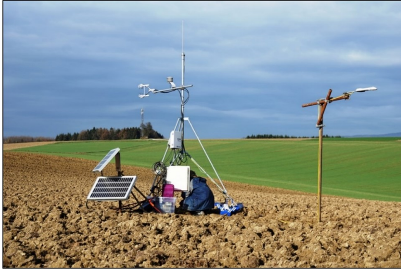
Fig. 4. Eddy covariance system (IRGASON) mounted on a 2.5 m tripod.
