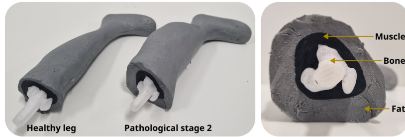
Figure 3: Healthy and pathological leg phantoms constituted by 3 layers: bone, muscle and fat.
