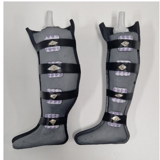
Figure 6: Anthropomorphic leg BIS measurement setup.
