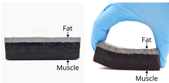
Figure 20: Connection between the muscle layer (black matter) and the layer of fat phantom (grey matter).
