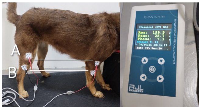
Figure 1. (Left) Placement of voltage electrodes (A), current electrodes (B). (Right) Values of R, Xc, and PhA provided by the BIA device. Source: own elaboration.
