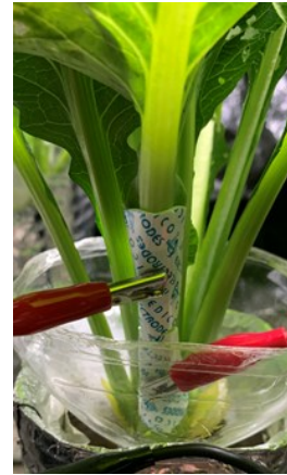
Fig. 1. Experimental setup for EIS measurements. Two ECG electrodes were noninvasively attached to the petiole of a Komatsuna plant with an electrode separation of approximately 25 mm, enabling in situ impedance measurements without tissue penetration.
