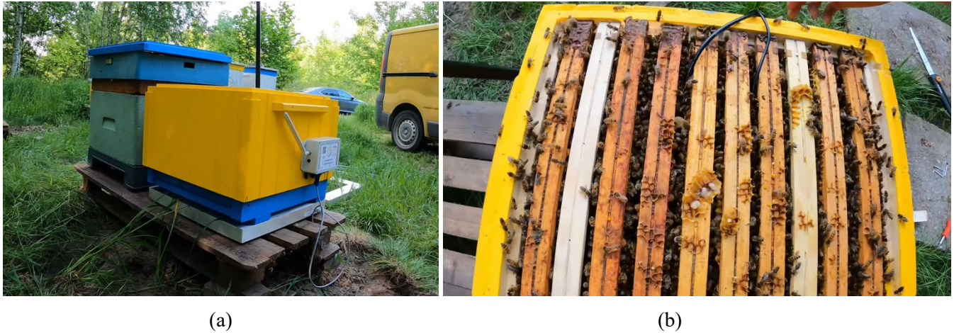
Fig. 2. Physical installation of the BeeHUB sensing system. (a) BeeHUB Queen device and hive-scale platform mounted underneath the beehive for continuous load-cell-based weight measurement. (b) Placement of the internal temperature, humidity, and acoustic sensing module between hive frames to capture representative microclimatic and acoustic conditions inside the colon.
