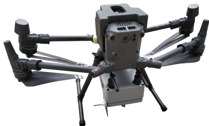
Fig. 2. Measurement device Pixla 1 mounted on a UAV (DJI Matrice 300)
