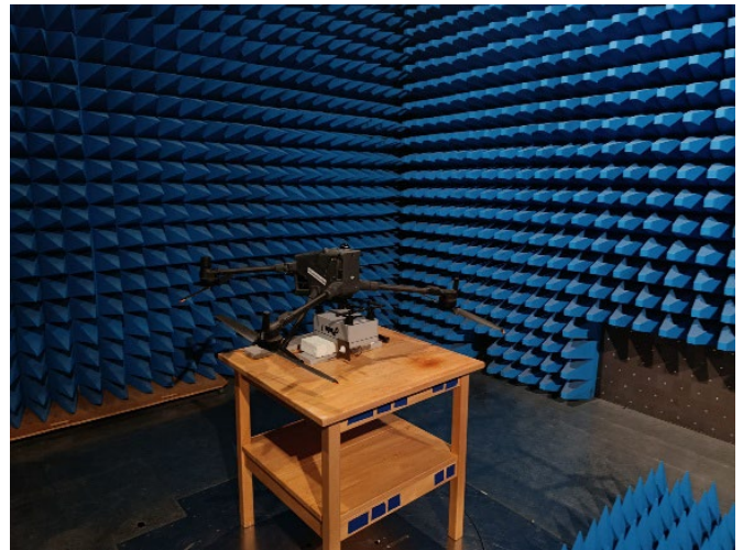
Fig. 11. Experimental radiation pattern measurement of Pixla 1 mounted on a UAV in the EMC semi-anechoic chamber
