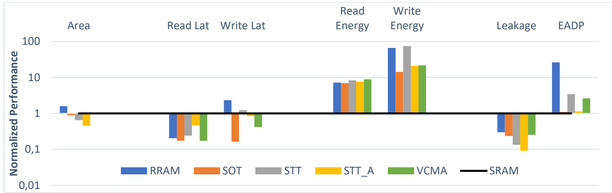
Fig. 9. Comparing non-volatile caches normalized average performance with SRAM as baseline
