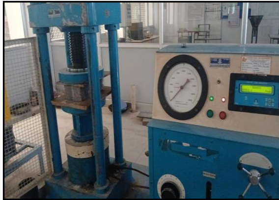
Figure 10. Compression testing of paver block
