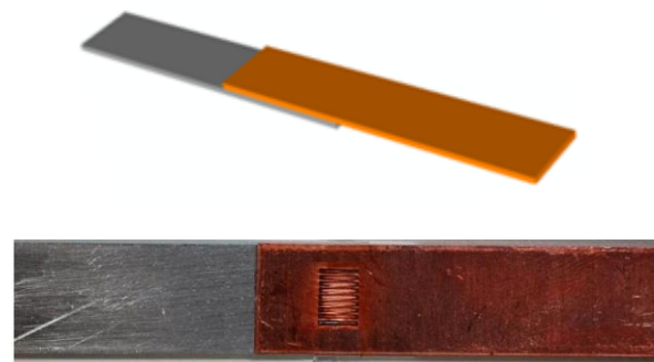
Figure 11. Pictorial and photograph of Al/Cu lap joint sample
