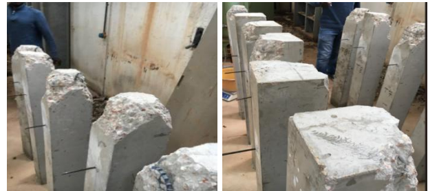
Figure 7. Column Samples after Failure
