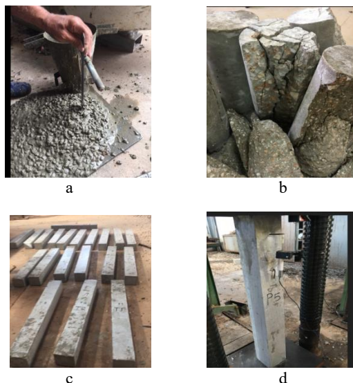
Figure 6.a) Concrete of Testing Columns, b) Cylindrical Specimens Post-testing, c) Column Samples under Curing, and d) Typical Column under Testing
