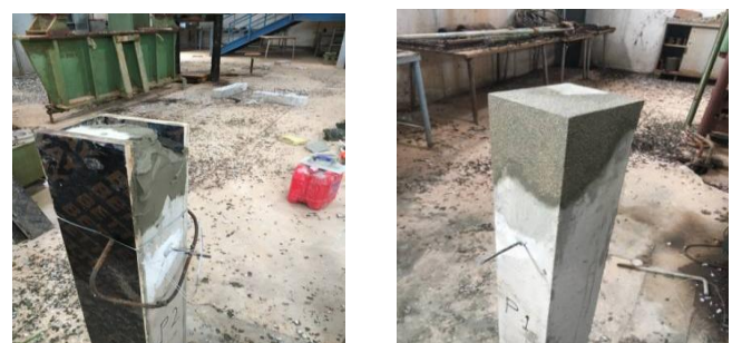
Figure 8. Smoothing and Finishing of Tested Column surfaces
