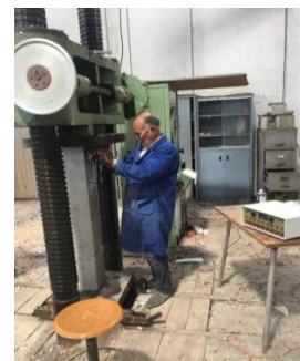
Figure 1. 300-Ton capacity compressive testing machine
