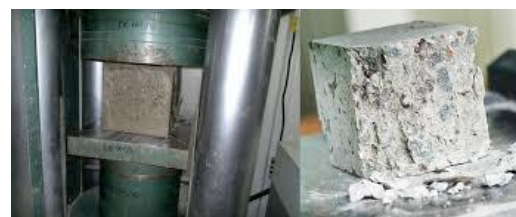
Figure 7. Pictorial view of cube specimen under compression
