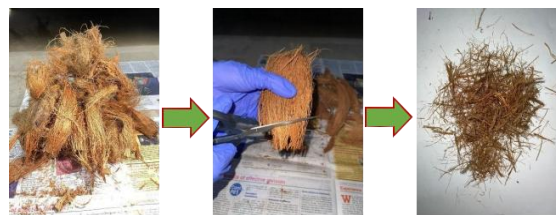
Figure 2. Process of conversion of coconut husks into desired fibers
