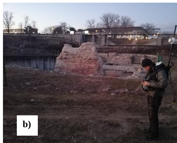
Figure 9. a) Dynamic penetration test (SPT) execution (at the upper side of the figure), b) Geophysical data collection with the GSM-19 magnetometer (down side of the figure)
