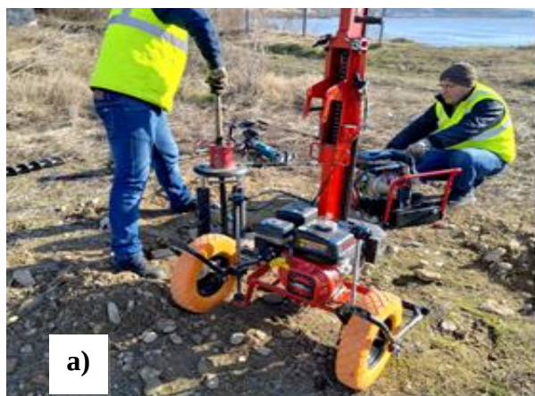
Figure 9. a) Dynamic penetration test (SPT) execution (at the upper side of the figure), b) Geophysical data collection with the GSM-19 magnetometer (down side of the figure)
