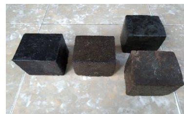
Figure 1. The Plastic Wall Block (PWB) Samples
