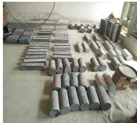
Figure 5. The casted cylinder and beams
