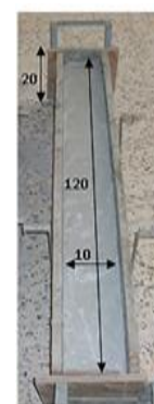
Figure 5. Prismatic molds used [10 \times 20 \times 120] \text{ cm}^3
