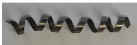
Figure 12. Fibers used L=6 \text{ cm} with 6 undulations
