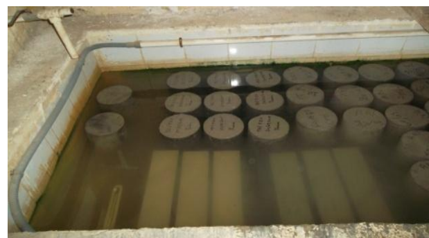
Figure 11. Samples kept in a bath at 20°C for 28-days
