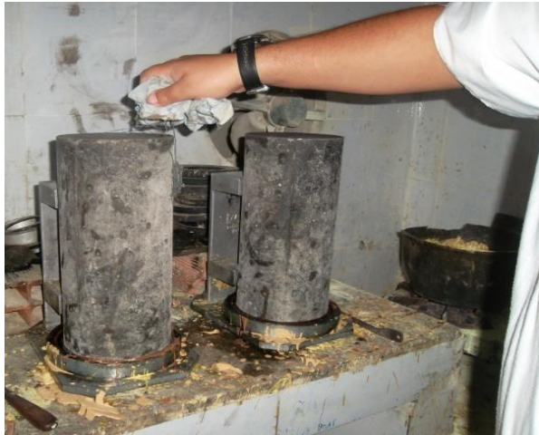
Figure 12. Surfacing of the specimen with sulfur and sand
