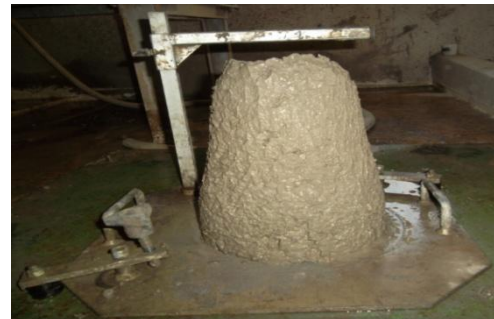
Figure 9. Slump measurement of concrete with Abrams cone
