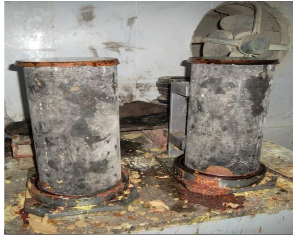
Figure 12. Surfacing of the specimen with sulfur and sand
