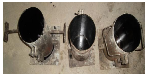
Figure 6. Lubricated Cylindrical test moulds
