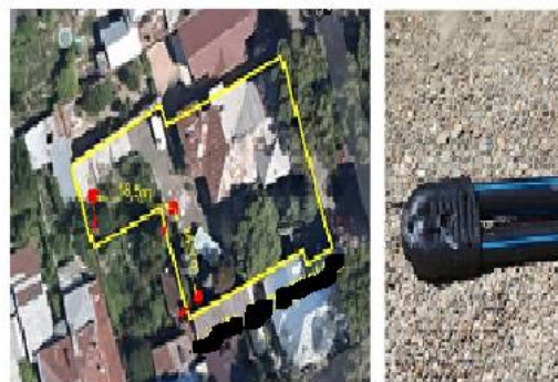
Figure 2. Location of heat exchangers with soil/ The tube protection. The position of drillings (three) is marked with red. The scale is 1:500
