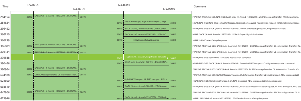
Figure 6: Flow graph: Network messages from a UE connecting to a 5G (NR) network. UE, user equipment.
