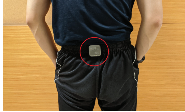
(b) Placement of the IMU on the test subject.
