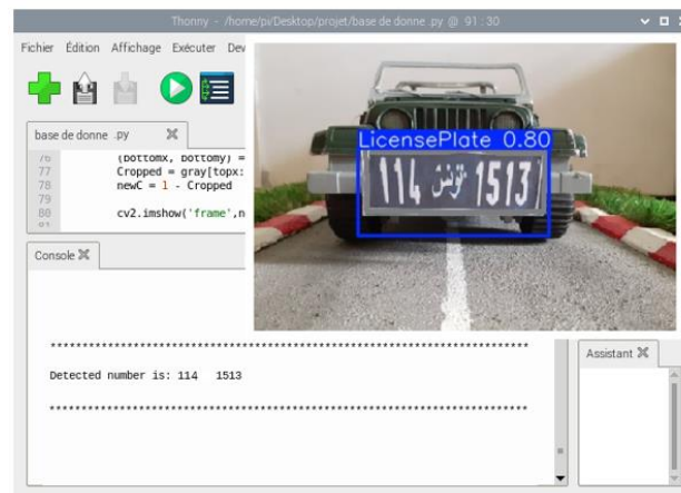
Figure 4. ANPR on Raspberry Pi.
