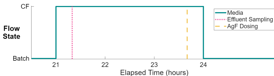
Figure 2. Daily operational timeline for the SMBR. Hours 0-21 are left off of the figure for ease of interpretation (batch phase with no sampling/dosing occurring). CF= continuous flow.
