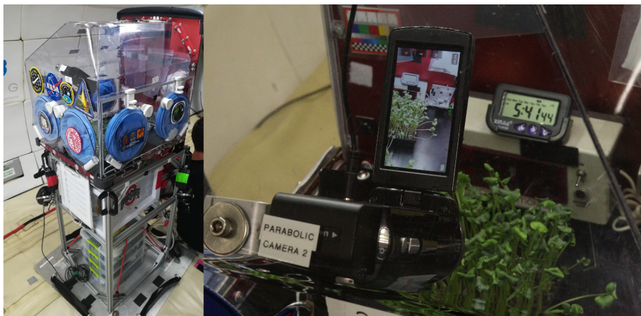
Figure 3. Experimental setup within the ZeroG aircraft. Left: overview of the glovebox in its flight configuration within the aircraft. Right: a view inside the glovebox showing one of the two cameras filming the inside.
