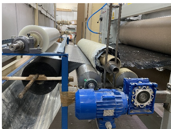
Figure 7. Continuous lamination process of the feather-wool nonwoven composite with compostable film and spunbond layers.
