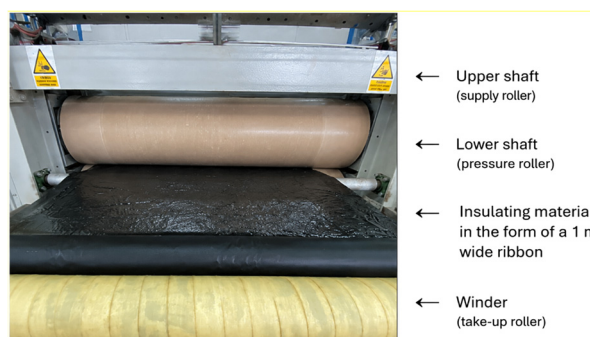
Figure 6. Two-roll calender used for continuous thermal bonding and lamination of the multilayer insulation composite.
