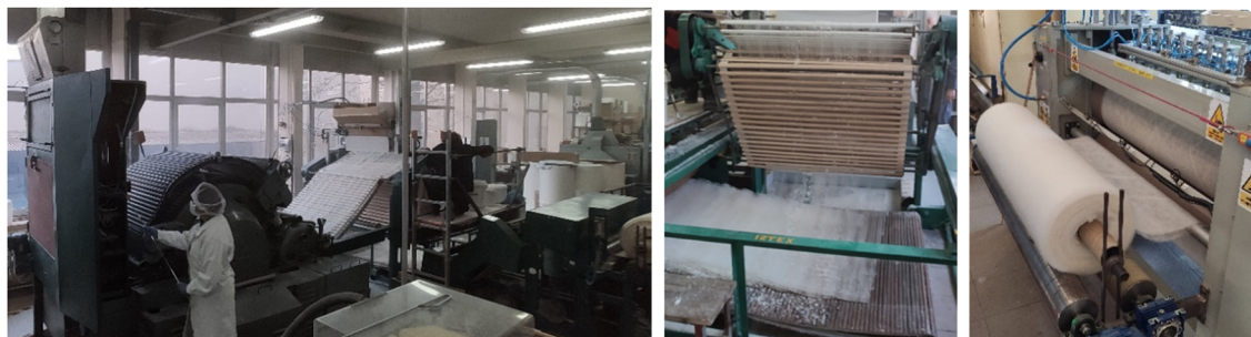
Figure 2. Complete process of nonwoven manufacturing by needle punching.
