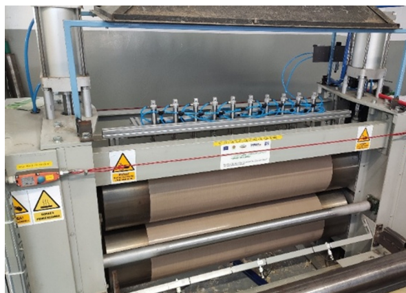
Figure 5. Infrared heating unit used for thermal consolidation of the feather-wool nonwoven composite prior to lamination.
