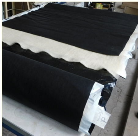
Figure 8. The layering of a composite intended for the construction of a beehive thermal insulation.
