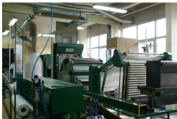
Figure 4. Needle-punching production line for nonwoven insulation using needle punching method.
