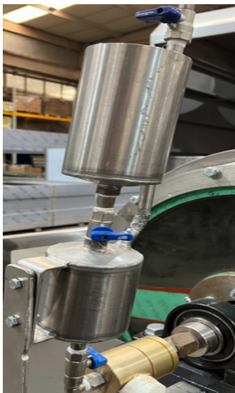
Fig. 2. Chemical dosing unit, and the set-up between the drum and dosing unit
