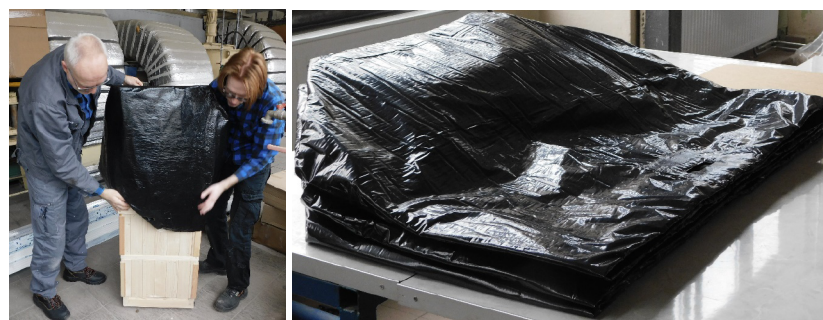
Fig. 3. Thermal insulation cover
