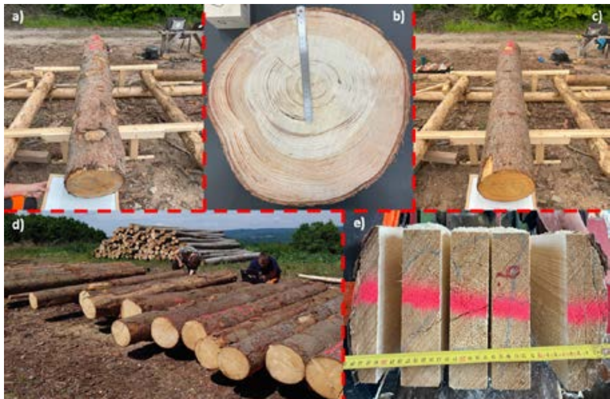
Fig. 1. Low-quality sawlog III.D (a); Sample for the determination of the moisture content (b); High-quality sawlog III.A (c); Measuring area at the Sawmill Olomučany (d); Cant sawing with a resulting 3 centre boards 50 × 160 × 3,000 mm (e).
