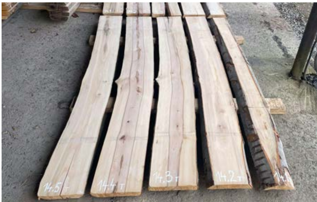
Fig. 3. Labelling of sawn timber from a beech log prior to CT scanning.
