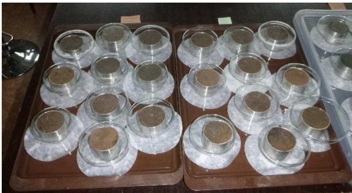
Fig. 2. Experimental rings filled with soil samples during passive capillary drainage.
