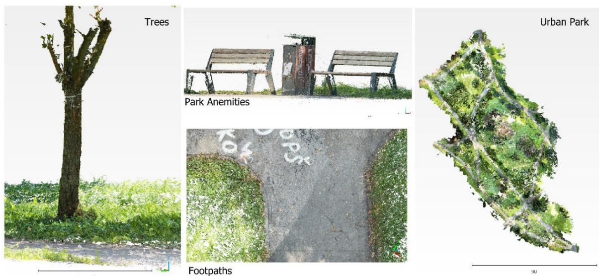
Fig. 6. Point cloud visualization.
