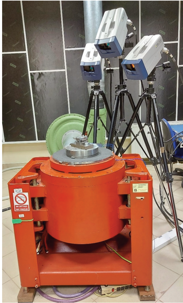
Figure 3. Test stand: E-390 shaker and heads of the PSV 500 3D scanning vibrometer.
