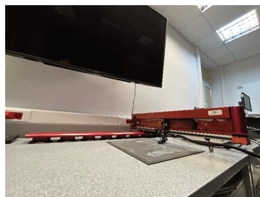
Figure 7. Components of MAUS V system. PC (a) and track with trolley, arm and sensor (b).
