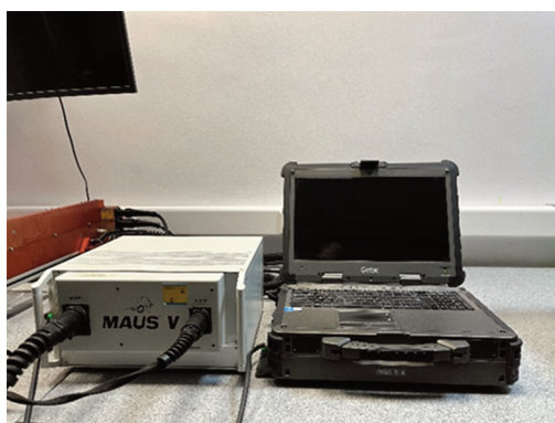
Figure 7. Components of MAUS V system. PC (a) and track with trolley, arm and sensor (b).
