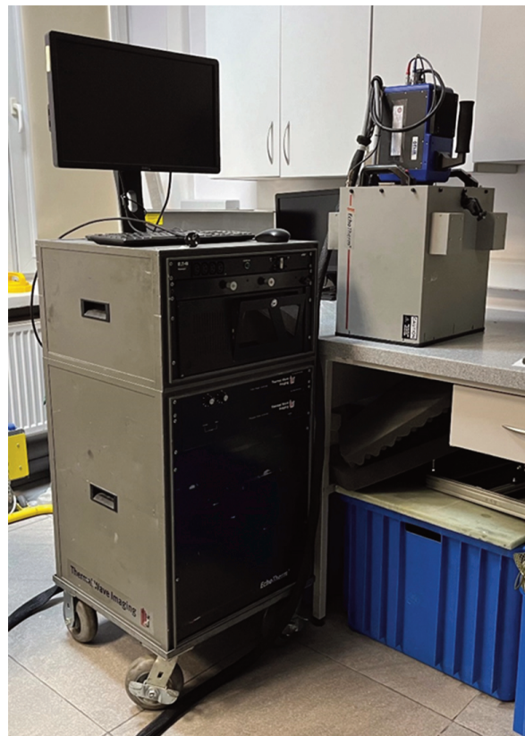
Figure 6. EchoTerm® Thermal Wave Imaging system used to collect TT data images.
