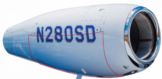
Figure 14. Honeywell HTF7000 nacelle. The contour of the tested part is marked with a red line. Original image source: Safran Group (2021).
