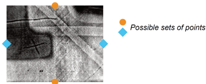
Figure 10. Possible sets of points that must be localized on both the 3D CAD model and its real counterpart to correctly position TT data on the model.
