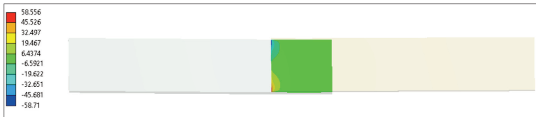
Figure 17. End of time, residual shear stress. Weld area plot, aluminum surface (20°C→240°C→20°C).
