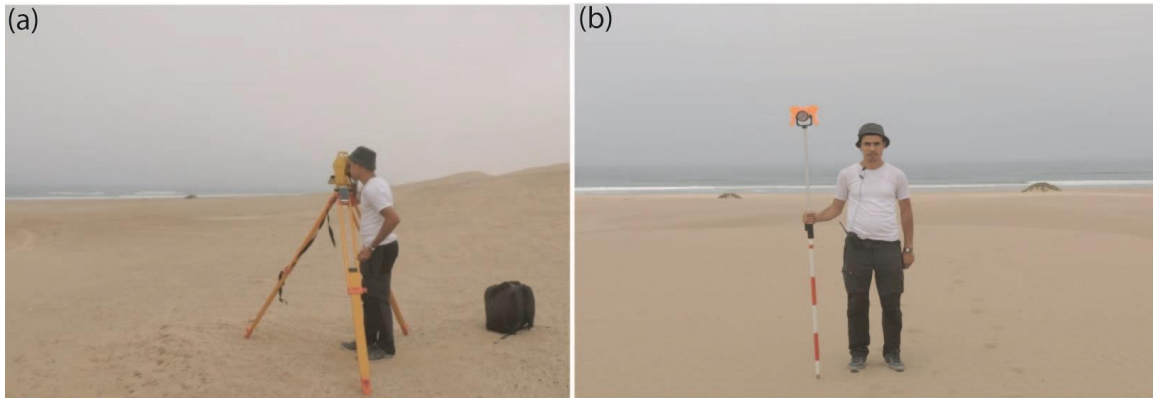
Fig. 4. Topographic survey instrument(a) Setup of the SOUTH NTS-375R electronic total station. (b) The rod and reflective target used for the survey
