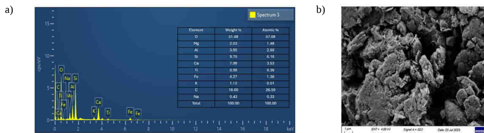
Fig. 4. a) EDX of alum sludge, b) SEM of alum sludge
