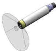
Fig. 2. The OBS-3+ emitted light and detector cones
